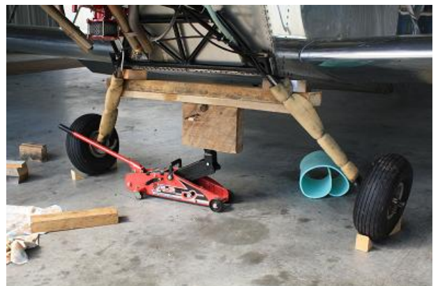
A trolley jack takes the weight off u/c legs.
