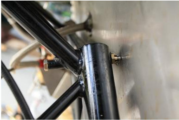
The new motor mount bolt with castellated nut.
