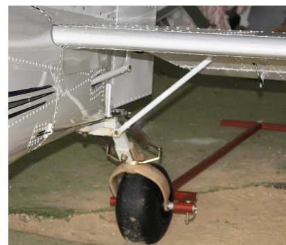
The elevator brace to be faired.
