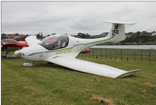
Zephyr ZK-ZFR with collapsed undercarriage.
