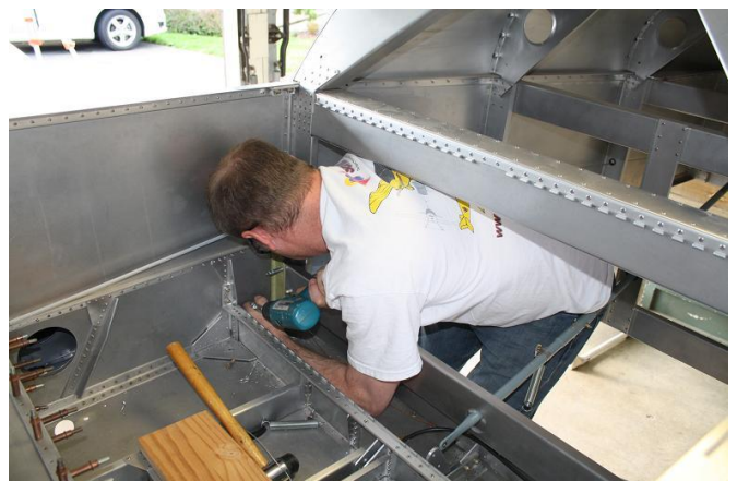
Drilling the rear spar bolt holes.
