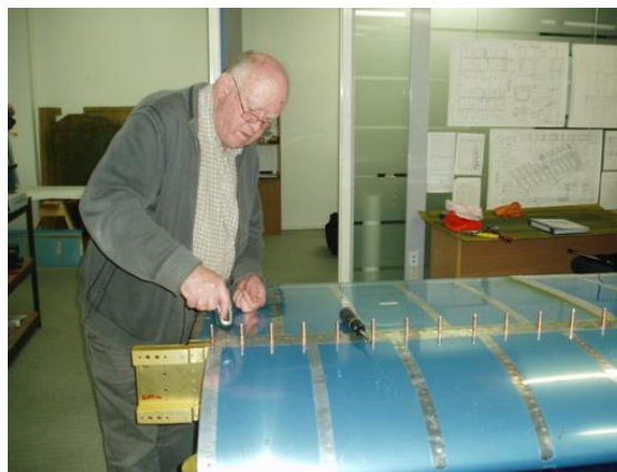
Attaching the fuel tank to the left wing
