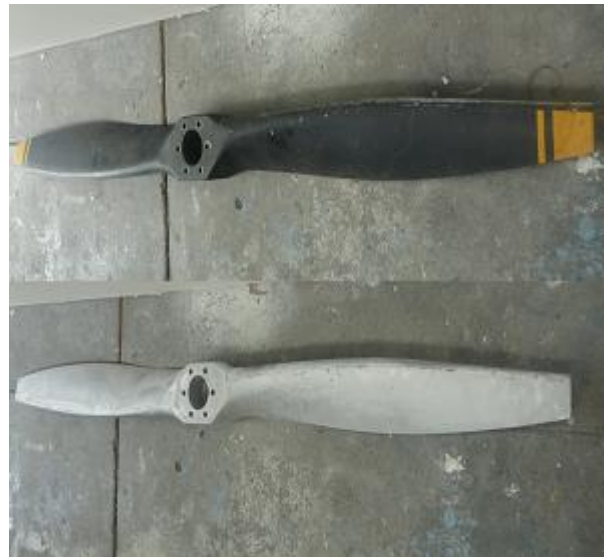
Example of Prop before and after SodaBasting
