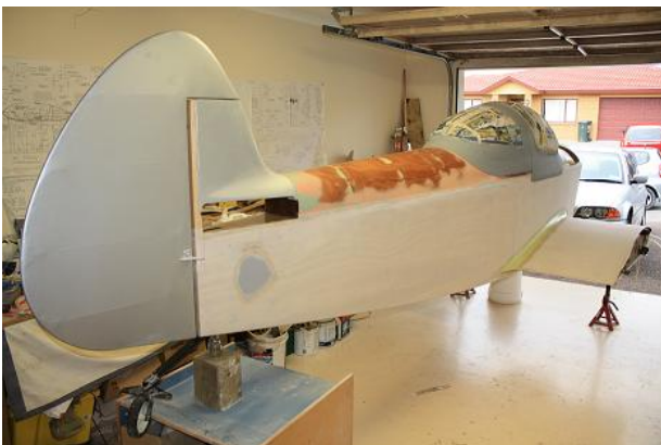
The Seconite fabric on the fuselage
