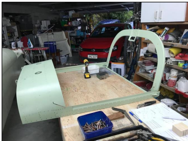
Canopy frame ready for installation
