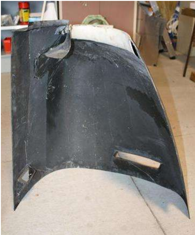
The Carbon Fibre cowls with the annular airflow moldings.
