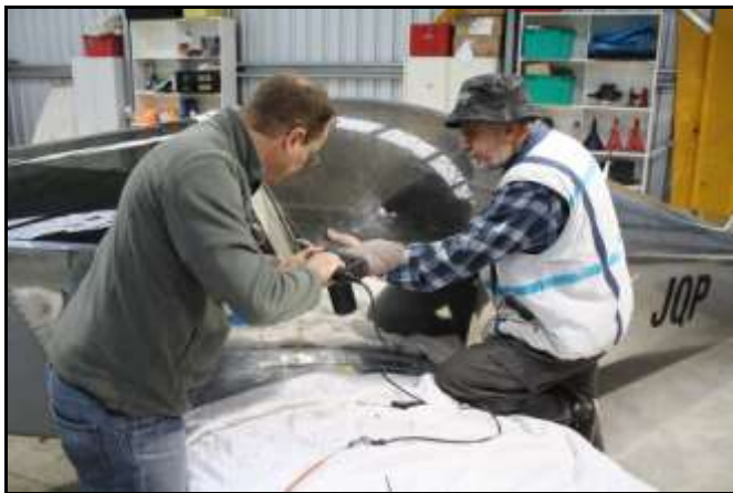
Finer adjustments with a smaller belt sander.
