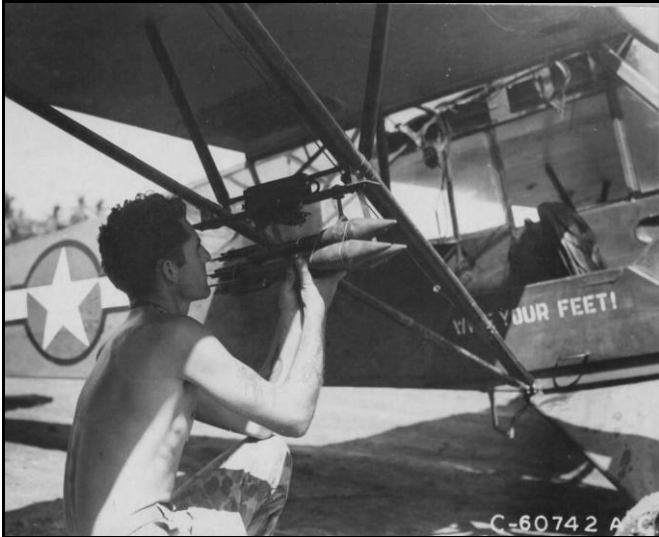
An improvised bomb shackle on an L-4 airplane flying in support of the 158 th Infantry. The bombs are bazooka shells. January 1945
