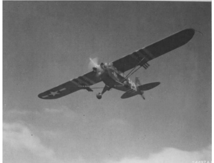
Piper Cub used by US Ground forces as an artillery liaison plane is shown in flight after its conversion into a rocket firing craft by installing bazookas.
