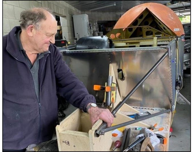
Mr Groves inspecting his welds
