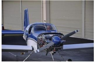
Phase 1 [of flight testing] will be completed without wheel fairings for ease of inspection and to increase drag to help with engine run-in and as a control for any heavy wing scenarios. Apparently, you can get a rate 1 turn if you get the fairing setup wrong. Just CAA and lots of paperwork to go then I'll be looking for something new. This one took 7 years but the next one won't take nearly as long, it doesn't come with a wing kit - but it will still fly!! Pat
