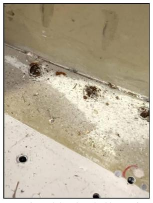
He was informed that there had been a fire on the first engine start due to a disconnected fuel line and a fire extinguisher was used to put the fire out. Obviously, the wrong type of extinguisher!
