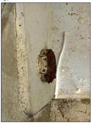
There was also a very fine powder throughout the interior of the aircraft, which I thought could have been fiberglass sanding residue. The corrosion looked like someone had spilled a bucket of acid inside the airplane, so we encouraged the owner to reach out to the builder.
