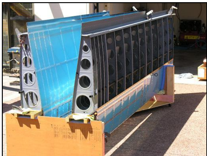
Built these and the empennage at home.
