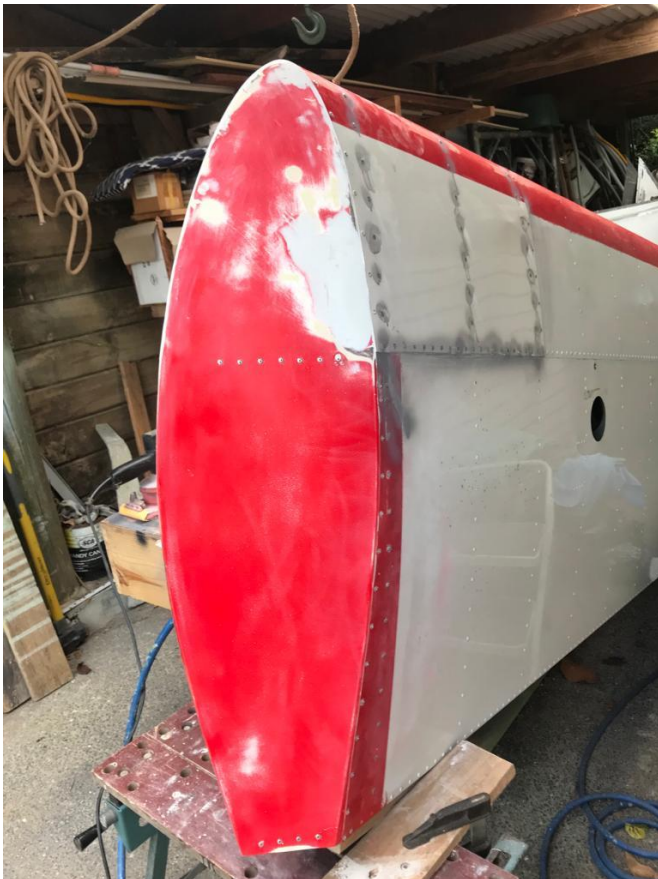
End cap ready for painting.
