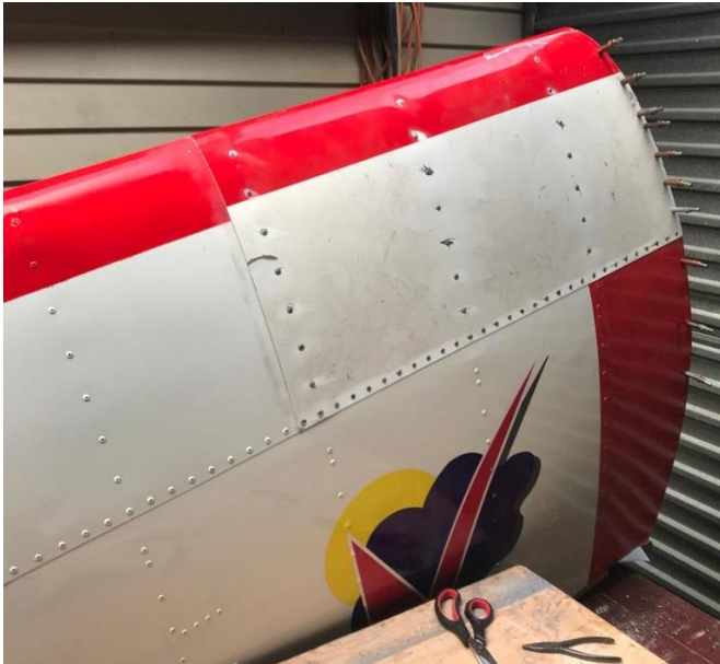
Leading edge riveted in place.
