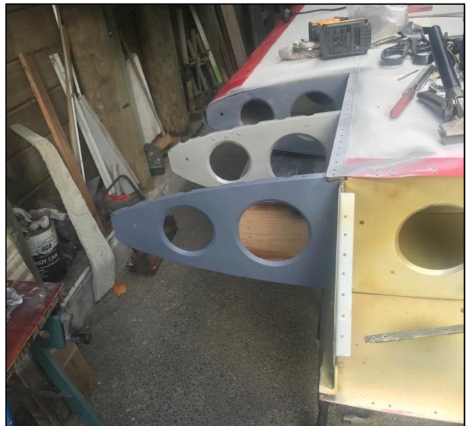
Starboard. Leading edge ribs replaced.
