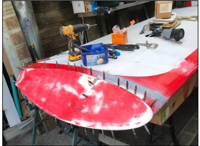
Fibreglass end cap repaired
