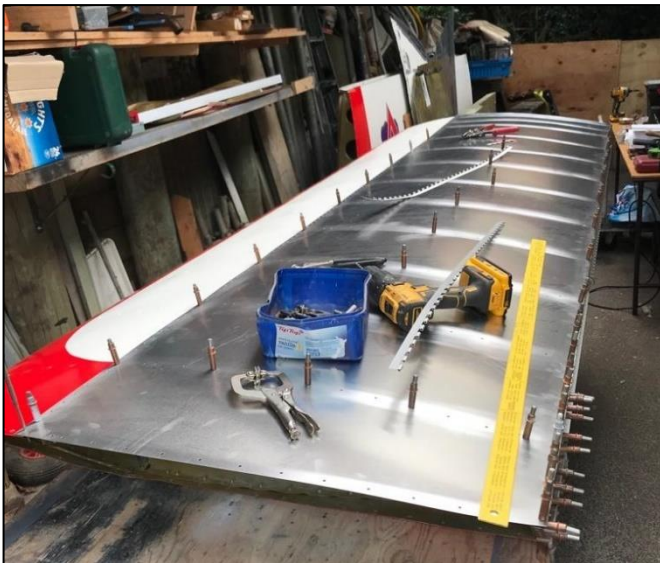
Port Wing. Top skin replaced
