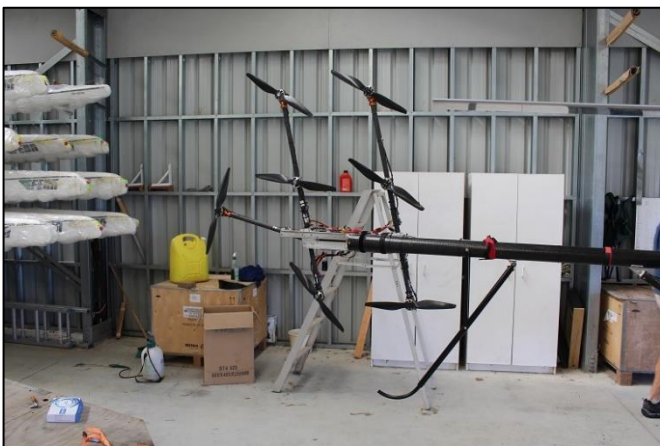
The sideways mounted drone tail rotors.
