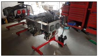
Martin supplied the old car battery from somewhere and build a neat little control panel so the engine can be wheeled out once a month or so and started to get the engine oil moving through the engine. Still quite a bit of work required to tidy up and replace wiring, plugs etc but it does at least go.
