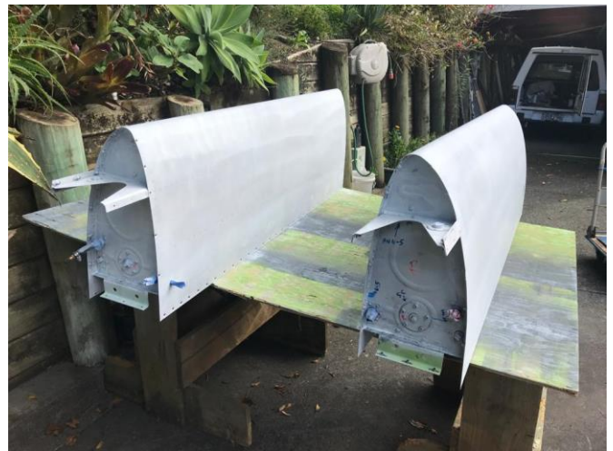
Tanks primed and ready for installation.
