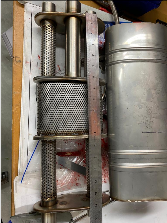
The inside of the muffler
