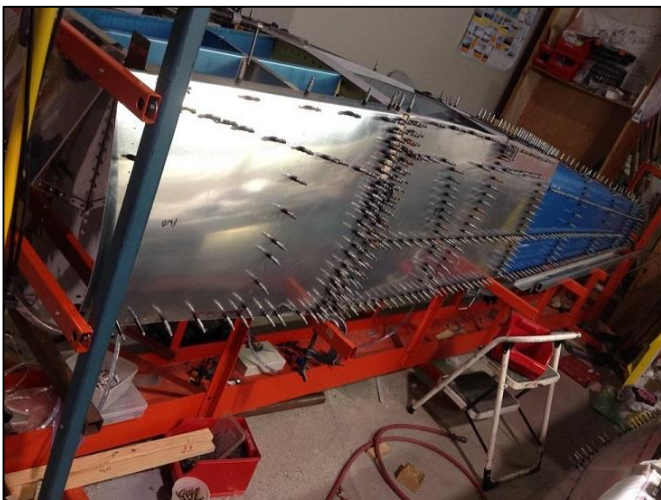
Sorting out the 0.040 fwd side skins - doing them in one piece rather than the usual two (with a join at the main spar) meant a bit more work and the use of a shrinker, but the end result should be worth it.
