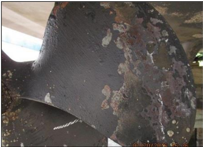
Paint blistered of propeller surfaces.
