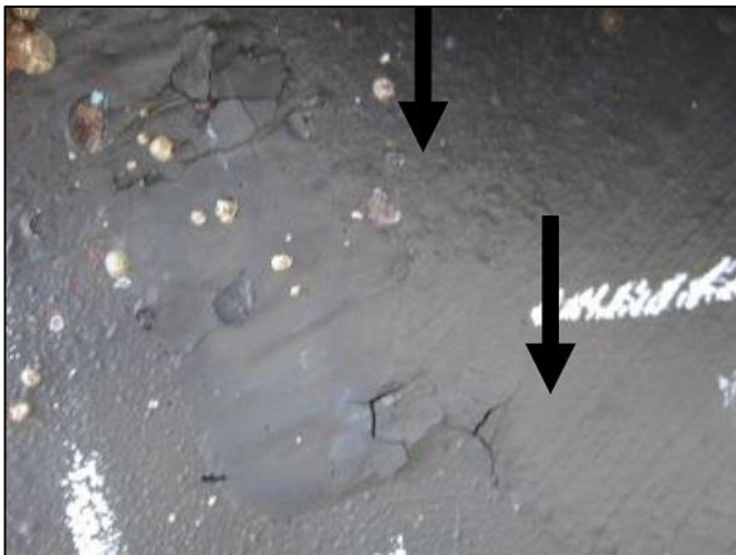
Paint blistered of propeller surfaces.
