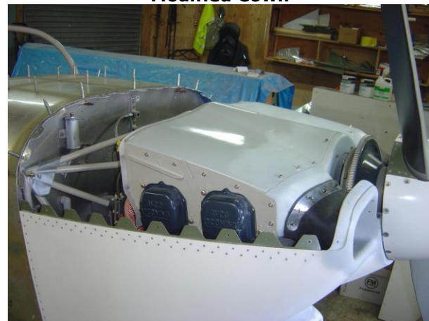
Close up of the engine plenum.
