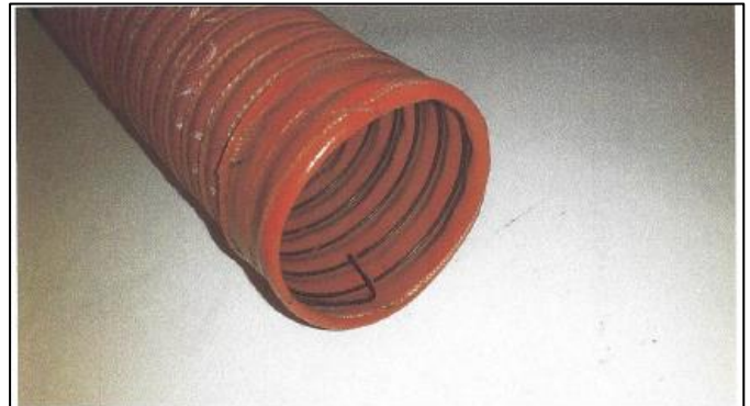
5. Cut back wire, bend 90 deg and tuck back into hose.
