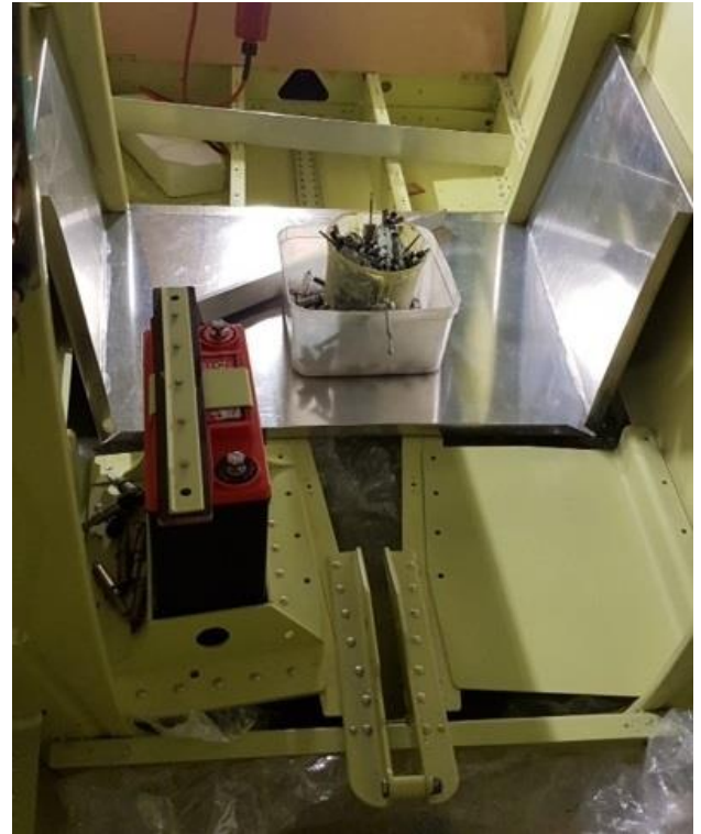
#2 Battery mount, ELT mounting plate, bellcrank mount.
