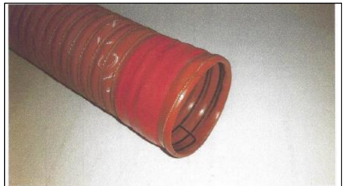
7. Wrap with self-amalgamating tape for protection against hose clamp pressure.
