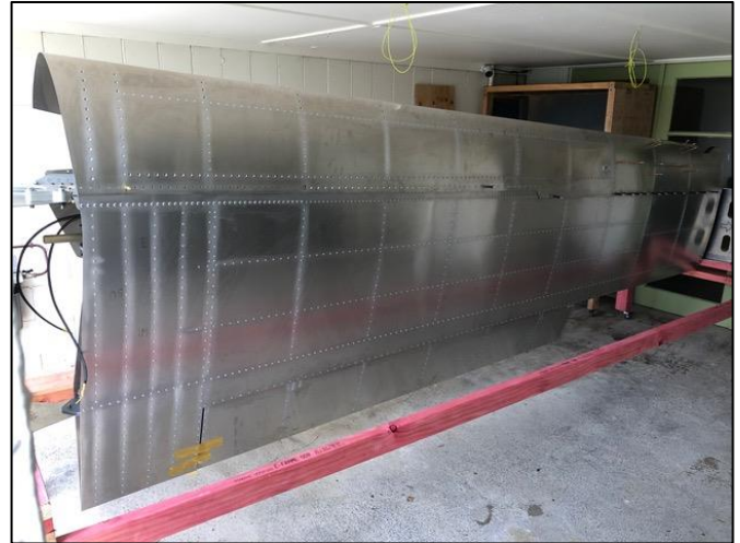
Completed right wing.
