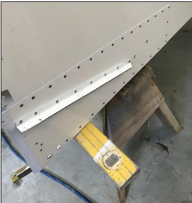
Repair at forward tail cone after flap damage
