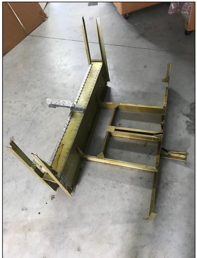
Wing spar tunnel after repair
