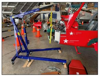
Actually, it's just one of the Van's Aircraft service bulletins that I have left to do to replace the nose gear, nose wheel fork, engine mount standoff, #1 and #2 exhausts, and carburettor clips and floats, but I'm doing them all now while I am still allowed to work on the aeroplane before it gets its C of A.
