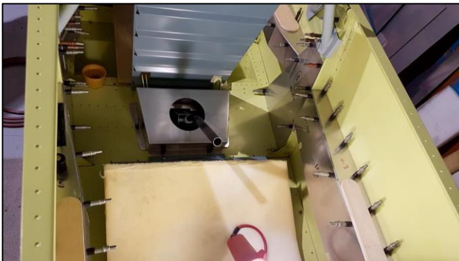
Passenger's control stick cover box being installed. This prevents the entry of FOD into the controls and is a place to mount ventilation and power outlets.
