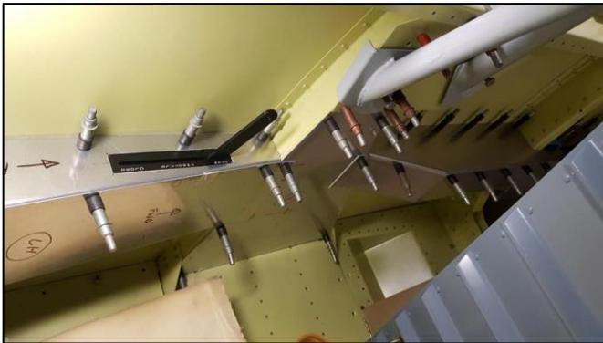
Passenger's control stick cover box being installed. This prevents the entry of FOD into the controls and is a place to mount ventilation and power outlets.
