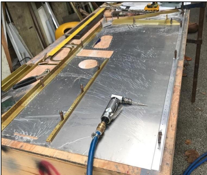
Match drilling existing parts.
