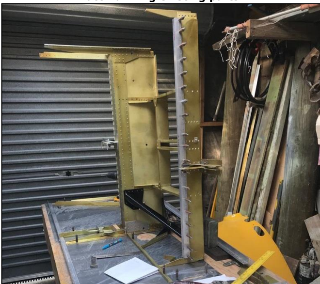
Replaced 0.032" seat angle with 1"x 1" x 1/8" angle.
