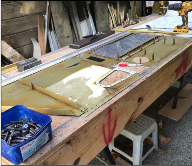
Checking set out with the existing damaged side skin.
