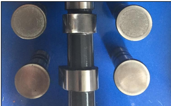
Pitted faces of lifters and worn cam.
